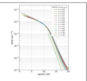
**Fig. 1**. EEDF in the sheath and at the wall of an argon plasma at 5 Torr (666 Pa) for a plasma density at the sheath boundary of  $10^{11}$  cm<sup>-3</sup>. The sheath boundary is at X=0, the wall at X=1, with  $L_{sheath}$  denoting the sheath thickness.
